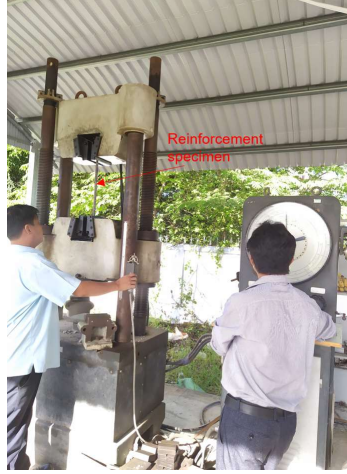
Fig.5 Tensile test of reinforcement specimen
