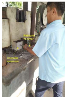
Fig.3 Rebound hammer test of concrete cube
