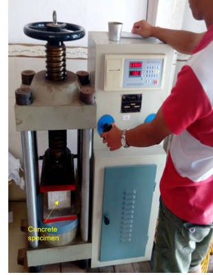
Fig.4 Compression test of concrete cube
