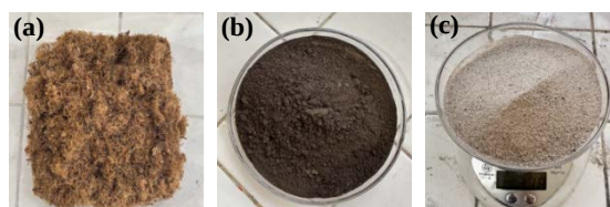
Fig. 2 Geopolymer component materials: (a) Bemban fiber; (b) fly ash; and (c) Silica sand
