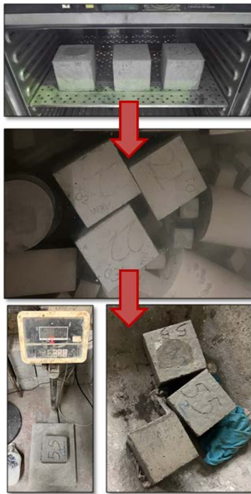
Fig. 4 Typical cycle in water absorption test.
