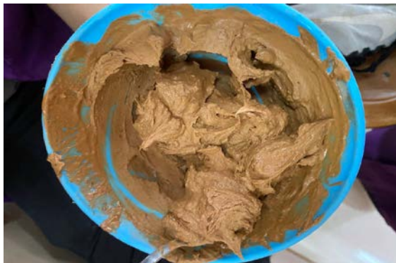
Fig 1. Soil Mixture Material to be Injected into The Borehole
