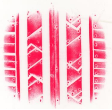
Fig. 4 Footprint of 205/65 R15 tire at an inflation pressure of 220 kPa and vertical force of 4,600 N
