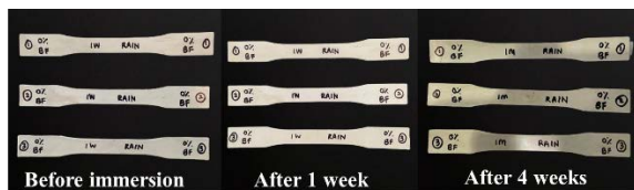
Fig.3 The 0% BF composite sample before and after immersion with rainwater solution (1 week and 4 week)
