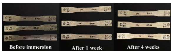
Fig.4 The 3% BF composite sample before and after immersion with rainwater solution (1 week and 4 week)
