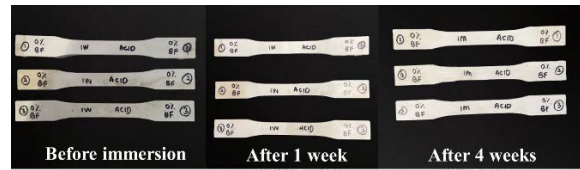
Fig.5 The 0% BF composite sample before and after immersion with acidic solution (1 week and 4 week)
