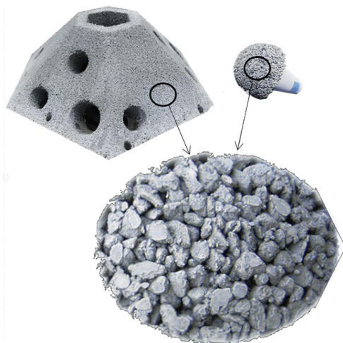
Fig. 6 Porous Substrate Structure
