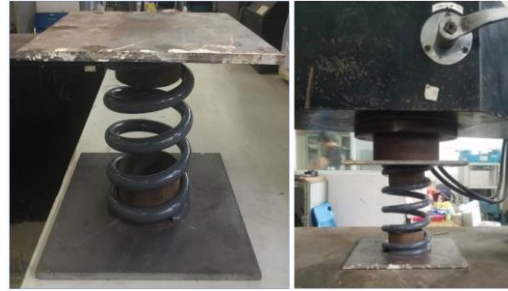
Fig. 5 Detail of a spring and stiffness test
