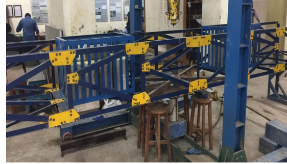
Fig. 3 External weight placement, each at a third and two-thirds span of the bridge specimen
