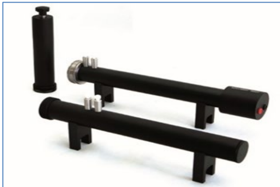
Fig. 3 BSWA SW477 impedance tube
