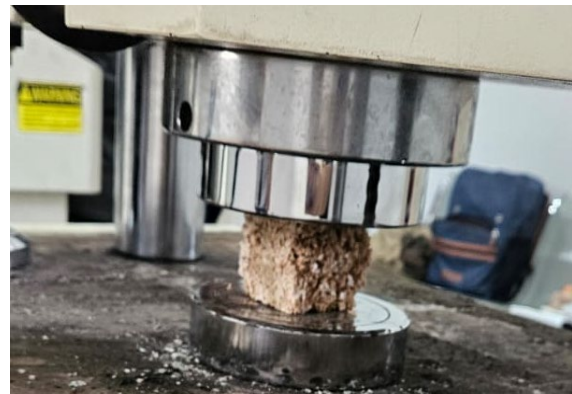
Fig.4 Compressive Strength Testing of Panels
