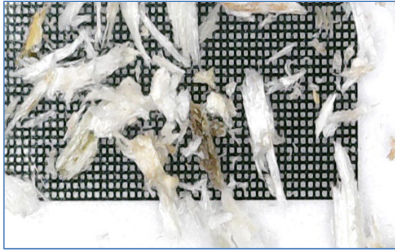
Fig. 2 Digital Microscope Image of Sawdust
