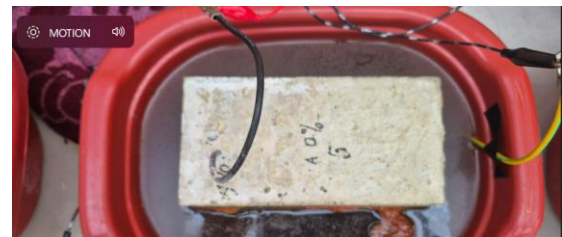
Fig. 15 Corrosion processes at 14 th days
