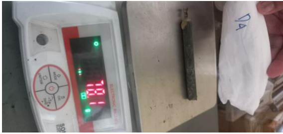
Fig. 17 Weighing of rust free steel bar
