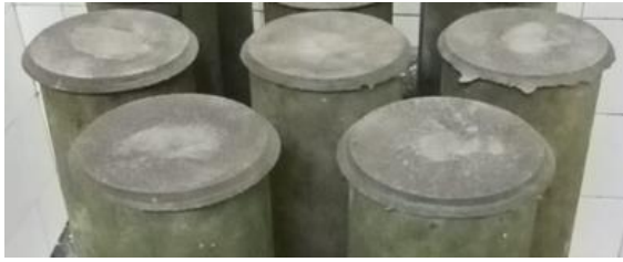
Fig. 11 Capping of concrete using sulfur
