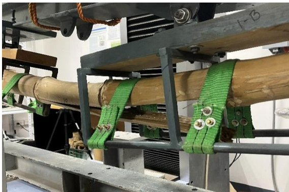
Fig. 6 Splitting along the bottom fiber
