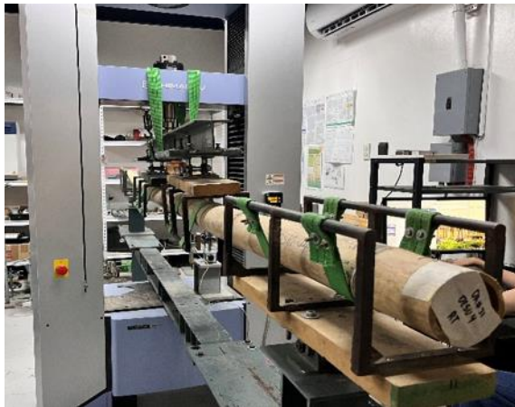
Fig. 1. Four-point bending test set up
