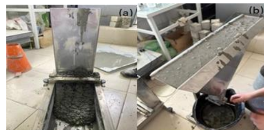
Fig. 1. Rheological testing of SCC: (a) L-box test; (b) V-funnel test
