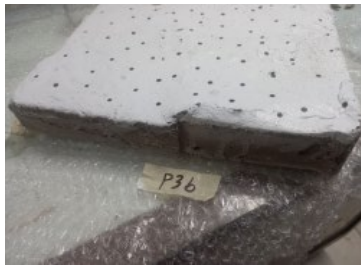
Fig.6 P3b wallet specimen showing the diagonal cracks and sliding shear failure of the material
