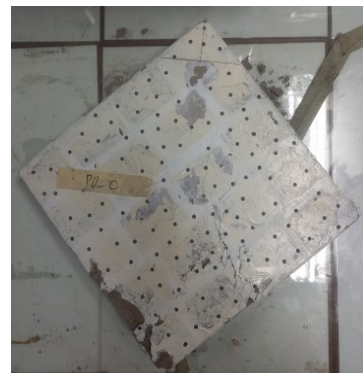
Fig.5 P0c wallet specimen showing the diagonal cracks after the test
