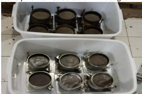
Fig. 1. Compacted specimens prepared for testing
