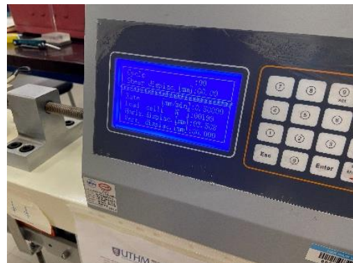
Fig. 10 Digital control panel for monitoring and operating the direct shear test
