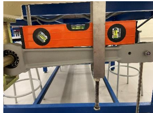
Fig. 9 Levelling and alignment of the shear box system
