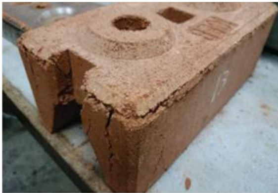
Fig. 9 Failure of individual full-size ICEB is characterized by brittle splitting and breaking
