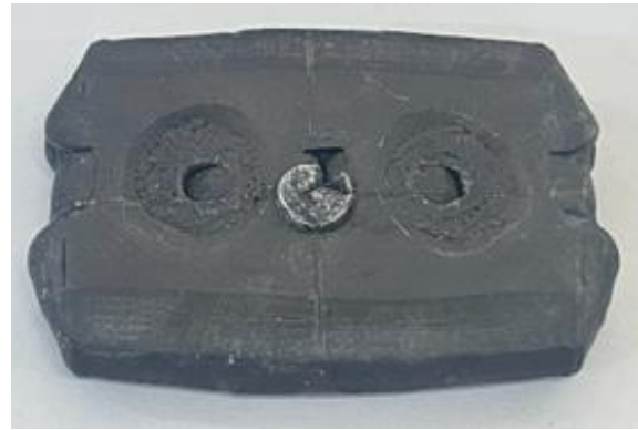
Fig. 10 Failure of individual scaled 3D-printed ICEB is characterized by more ductile form of crushing and squishing
