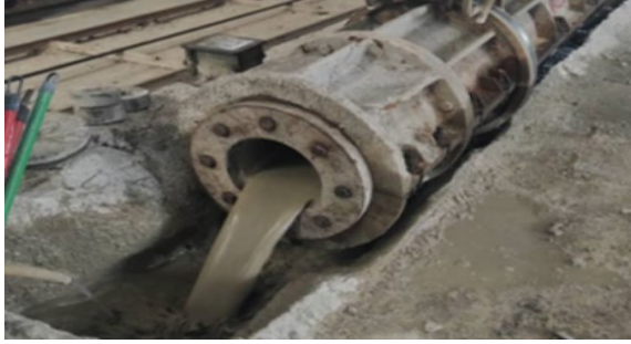
Fig. 1 CWS generated at the spun pile factory
