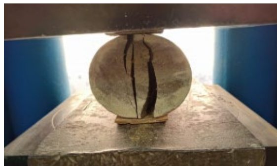
Fig. 5 Splitting tensile strength test
