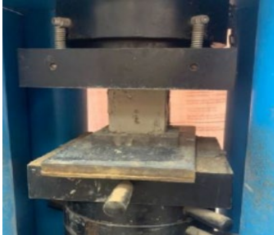
Fig. 4 Compressive strength test using compression testing machine
