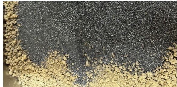
Fig.4 Mixing the dry soil with waste steel (WS).
