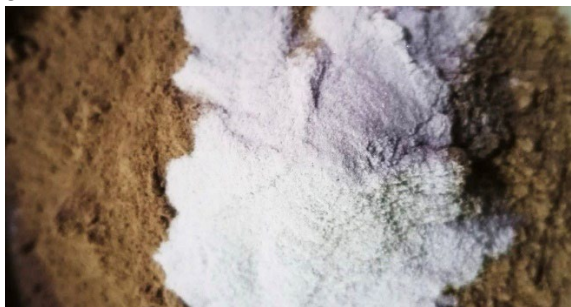
Fig.3 Mixing the dry soil with waste glass (WG).
