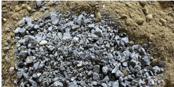
Fig.2 Mixing the dry soil with recycled crushed concrete (RC).
