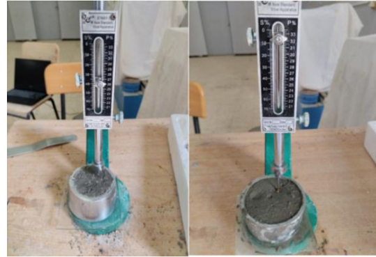
Fig. 2 Vicat apparatus used to determine setting time
