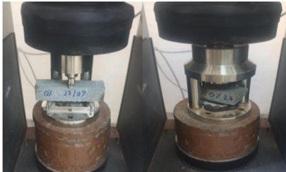
Fig. 4 testing flexural and compressive strength
