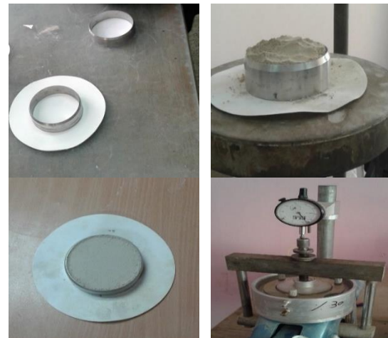
Fig.5 Soil preparation steps in single collapse test
