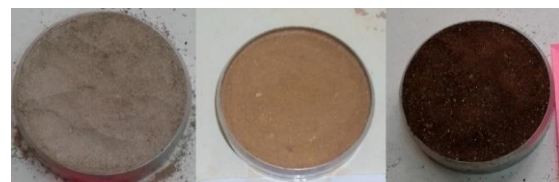
Fig.6 Soil samples stabilized with fly ash (left), bentonite (middle), and cutback asphalt (right) used in collapse tests
