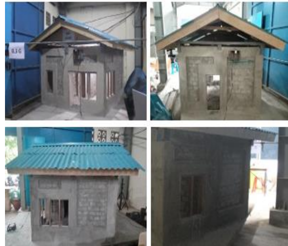
Fig.19 Specimen RH after testing under a 0.3g input
