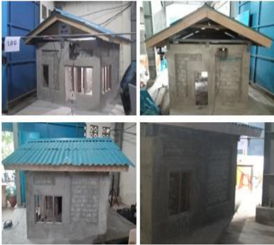
Fig.21 Specimen RH after testing under a 1.0g input motion
