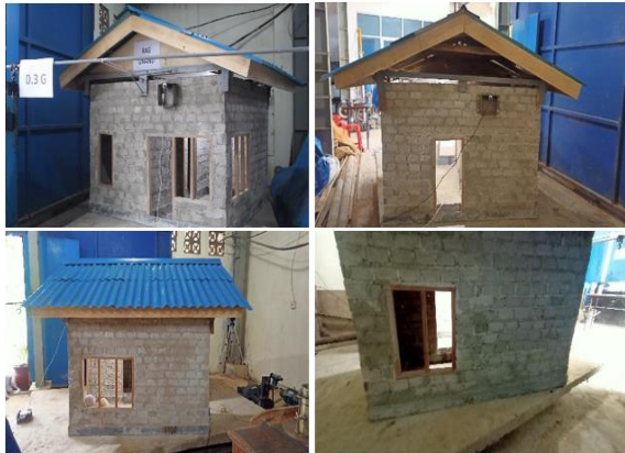
Fig.12 Specimen OH after testing under a 0.3g input motion
