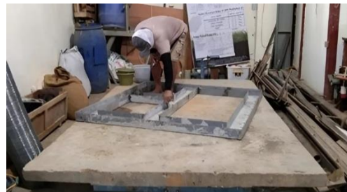
Fig.8 Installation of the U-plate on the shaking table
