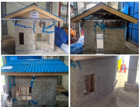
Fig.13 Specimen OH after testing under a 0.6g input motion
