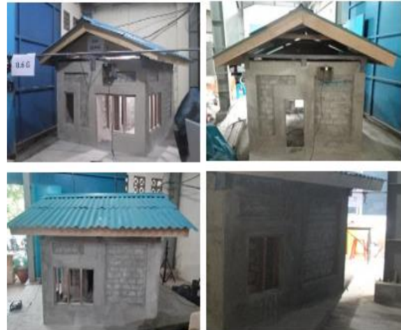
Fig.20 Specimen RH after testing under a 0.6g input motion
