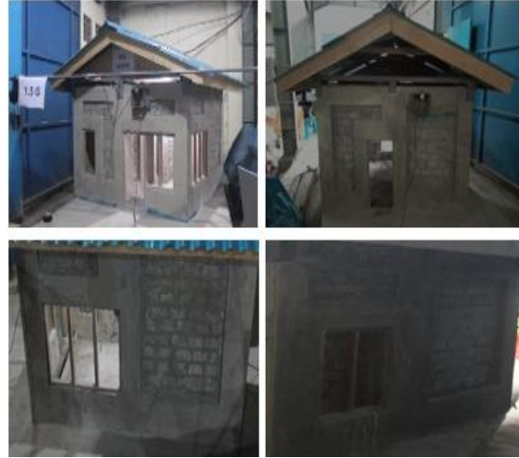
Fig.22 Specimen RH after testing under a 1.5g input motion
