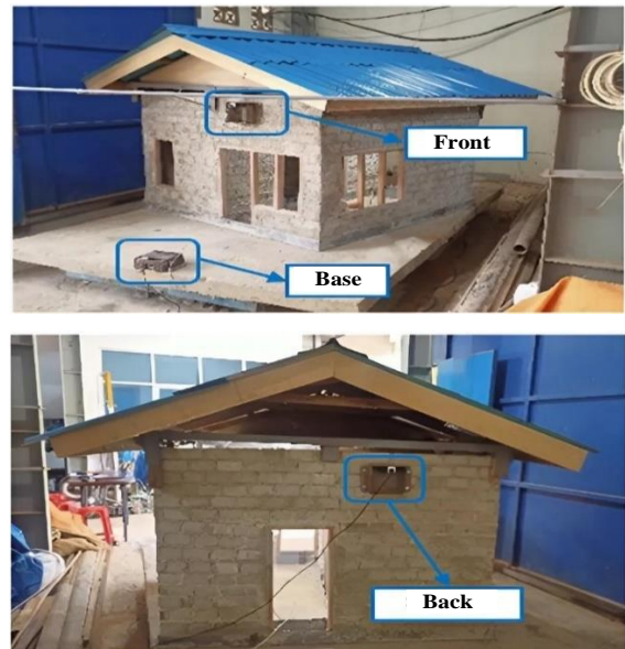
Fig.11 G-Trace tool sensor locations
