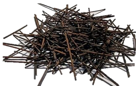
Fig.5 Steel fiber from waste tyres (4 cm in length)
