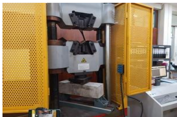
Fig.9 Flexural test on beam specimens
