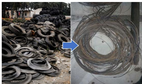
Fig.4 Steel fibers extracted from the waste tyres recycling process
