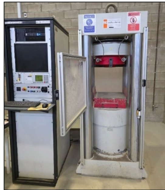
Fig. 2 Compression test set up
