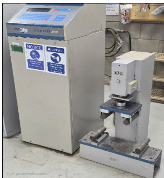
Fig. 3 Flexural test set up
