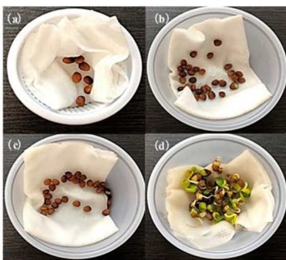
Fig. 18 Observation of radish sprouts after 10 day growth using (a) seawater, and the seawater treated with (b) raw mordenite zeolite (10 g/20 mL), (c) calcined Ca-Fe LDH (0.6 g), and (d) the mixture of raw mordenite zeolite (10 g) and Calcined Ca-Fe LDH (8.0 g)
